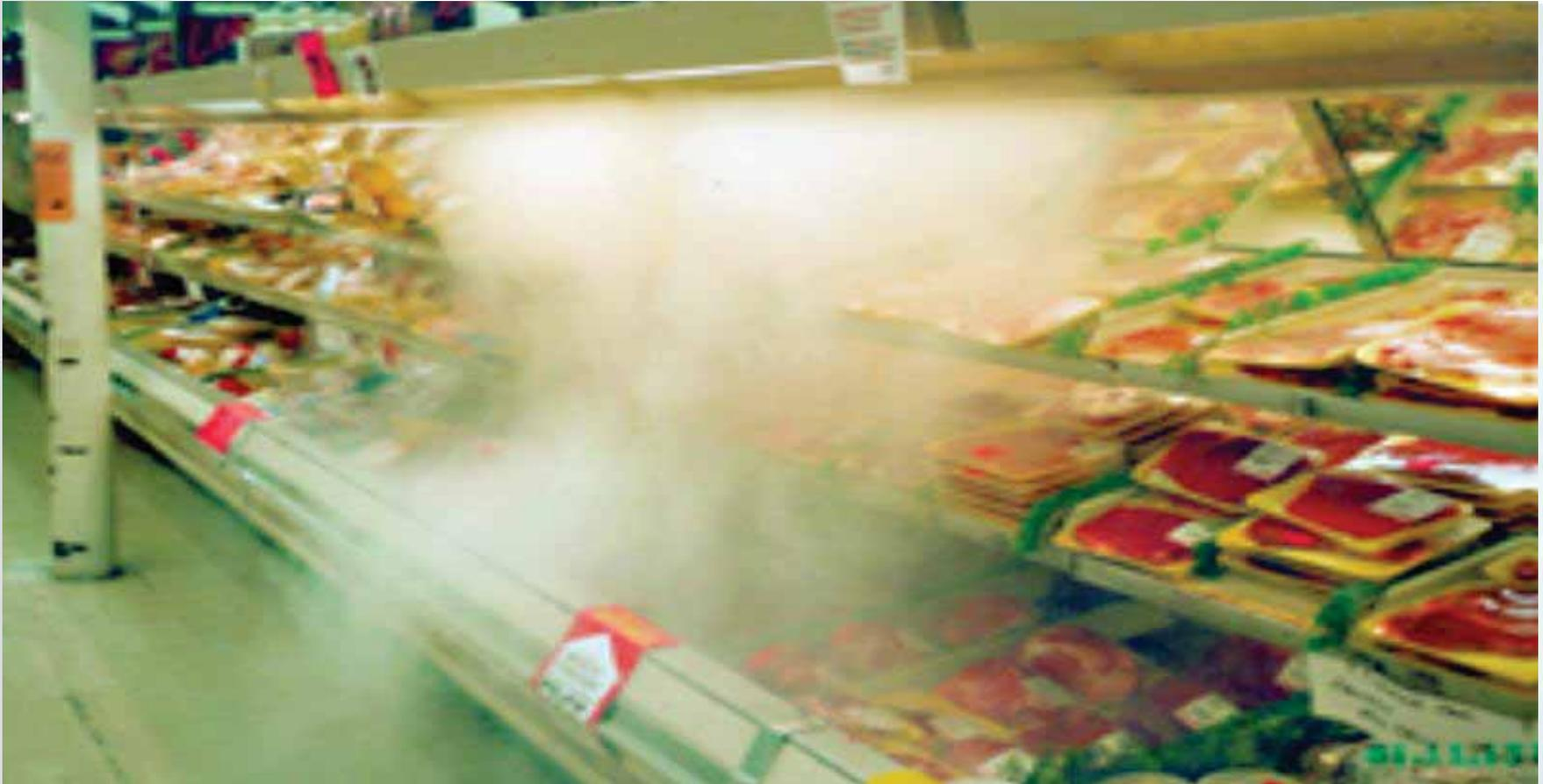
Smoke curtain demonstrates cold air spilling from supermarket open display case
