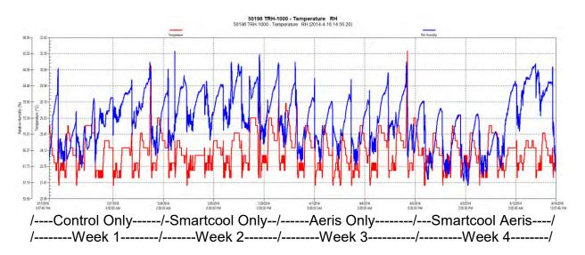
The above Graph shows the ability of the Smartcool system to reduce the effect of high humidity. The combined effect of Smartcool and Aeris on the relative humidity is obvious until the last 2 days when the region was directly affected by a cyclone where humidity was 100%. Regardless of this we were able to maintain internal humidity conditions close to the days when the relative humidity was much lower.
